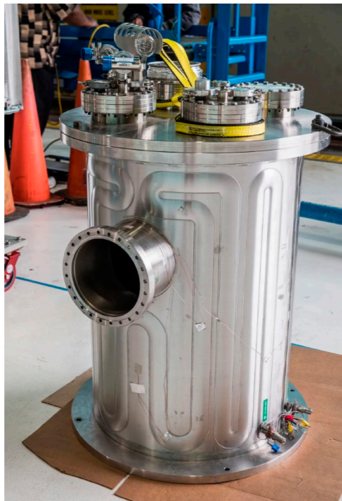
The assembled Kilopower experiment, enclosed in a vacuum chamber at NASA's Glenn Research Center. (Source: NASA)
