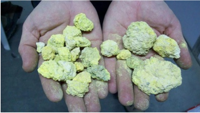
Carnotite mineralization from the Anit deposit at Blue Sky Uranium's Amarillo project in Argentina. Credit: Blue Sky Uranium.
